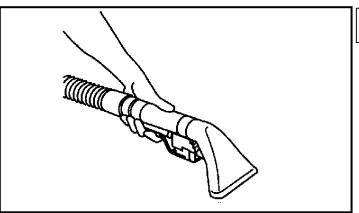
STEP Squeeze handle on accessory tool to begin cleaning.
